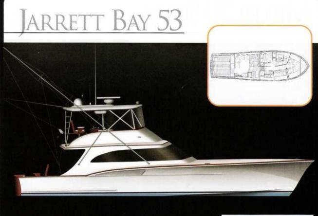
Jarrett Bay will achieve a boatbuilding milestone when it splashes Hull No. 50 this year. The benchmark boat is a 53-footer that features Jarrett Bay's proven low-profile hull design. Weighing in at only 49,000 pounds, the 53 features a refined running-gear configuration that maximizes available power. When equipped with a set of 1,200-hp MTU 8V 2000s, this 53 will flirt with a 35-knot cruise and top out at over 40 knots.
