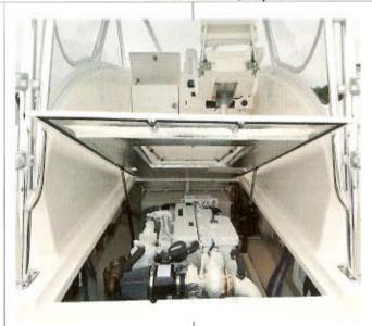
The cockpit sports a Carolina-style fish box/ livewell in the transom and two large below deck fish boxes. A central deck hatch offers access to fuel valves, jackshaft, bilge pump, and hydraulics for the power-assisted steering. The oil filters and Sepa fuel filters are positioned for ease of service.
