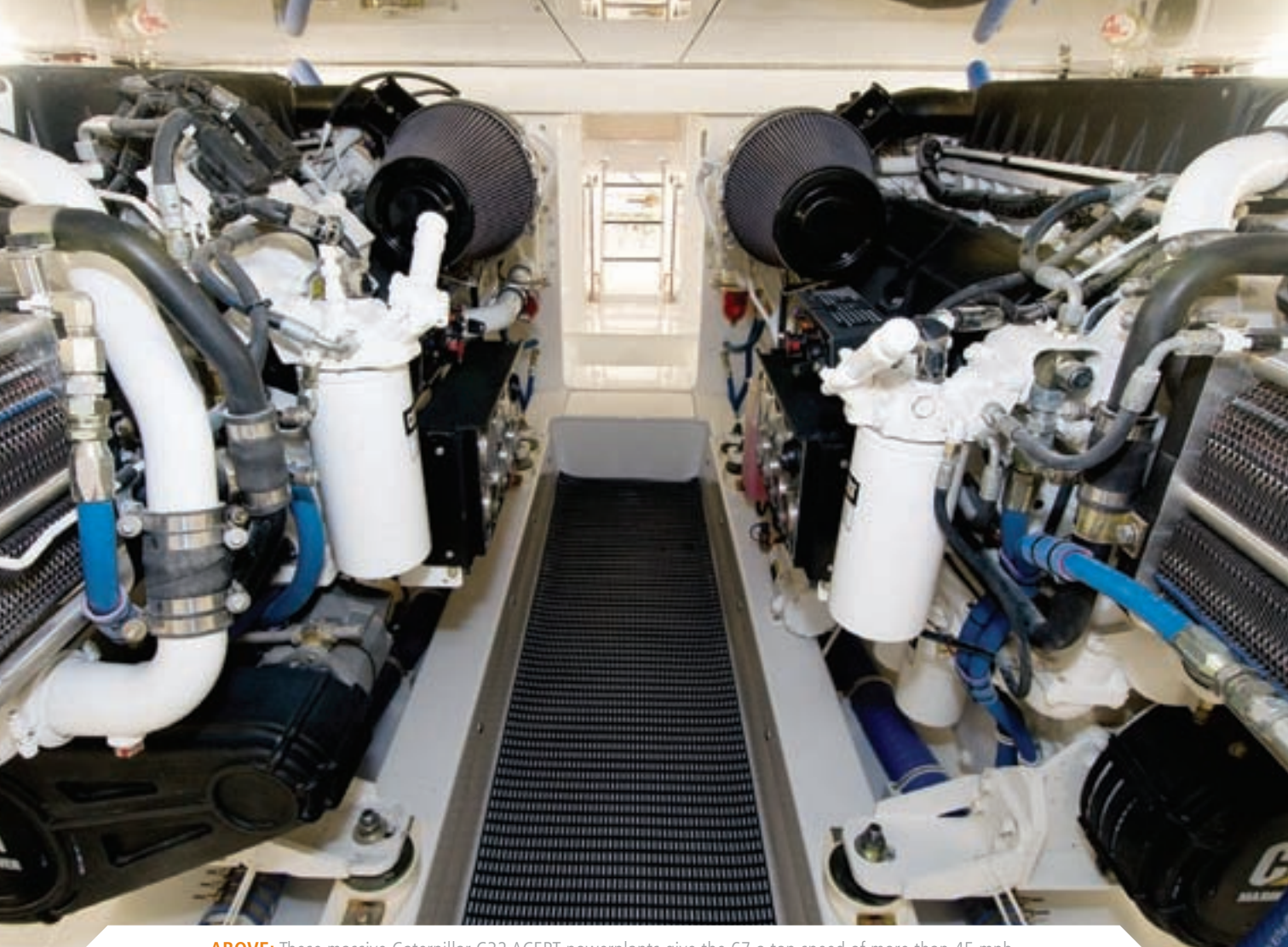
ABOVE: These massive Caterpillar C32 ACERT powerplants give the 67 a top speed of more than 45 mph.
