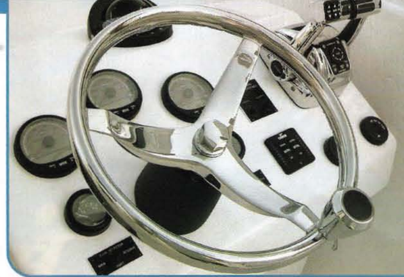
Mercury power-assist steering and electra-shift controls enable easy handling in close quarters and during performance-type maneuvers.
