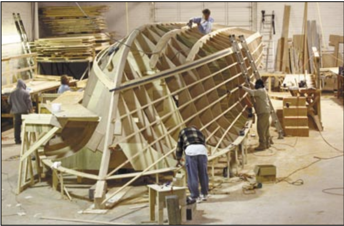
Craftsmen at Jarrett Bay Boatworks north of Beaufort work to quickly complete construction of a 46-foot sportfishing yacht for veteran NASCAR driver Jeff Burton. (Contributed photo by Danielle Johnston)
