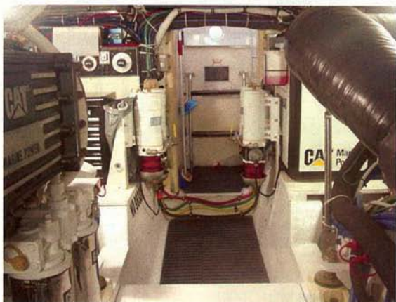
The HATTENUFF's new pair of CAT C-18's with ZF 550A gears.
