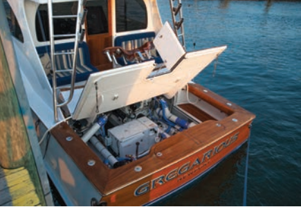
Your engine room has good access to service points? That's cute. The Jarrett Bay 43 brings new meaning to the phrase headroom in the ER with a hydraulically actuated cockpit.
