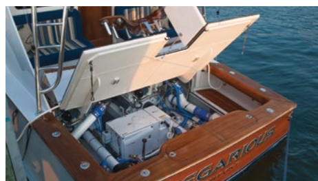
The teak cockpit sole has a secret too—lifting on hydraulics to reveal the aft portion of engine room
