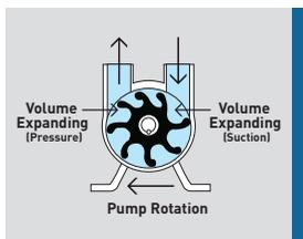
As a general rule, inspect the impeller and water pump assembly every year if operating in salt, brackish or turbid water, and replace if necessary. The debris in these waters acts like sandpaper. If operating in freshwater that is clear and clean, this interval may likely stretch to two seasons, provided no dry operation has occurred. Be sure to check your particular owner's manual for your outboard's specific service interval.
