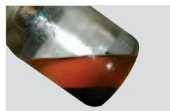
Ethanol, being alcohol, is also a powerful solvent that can loosen debris in your fuel tank and all the tanks and lines it was in before it got to you. Once in your outboard, this debris can cause everything from running issues to a no-start, no-run condition. That's no fun.
