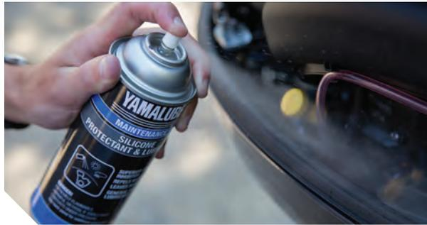
**Note:** Do not spray silicone on any oxygen (O<sub>2</sub>) sensors that your outboard may have.
