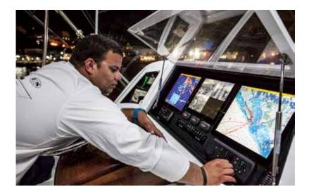
A clear acrylic panel provides good protection from the elements for an impressive lineup of multifunction displays, which are easily accessible for service or repair from the front or sides of the helm.
