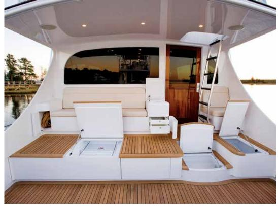
Perhaps the most significant innovation in modern sport-fishers is the mezzanine. This design feature provides not just comfortable seating for anglers and spectators, but also a wide variety of options for storage, refrigeration, and much more. Each location can be customized, while gas shocks hold open the lids for easier access. Even the mezzanine wing is useful real estate, housing speakers or even additional electronics displays.
