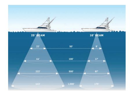
Early chirp sonars had only narrow-beam transducers, which offered high target separation but missed fish that captains were accustomed to seeing in wider beams. Choose the transducer that suits your style.
