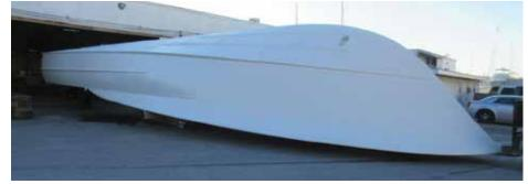
This boat is ready for a new owner to customize every part of her layout including interior and engines, or follow the tournament-winning specs of the 64' Hull #59 "Builder's Choice"! The exterior and interior of Hull #65 have been completely glassed, including the prop tunnels and stringers. And the network of framing down forward that will reside below the cabin floor has begun.
